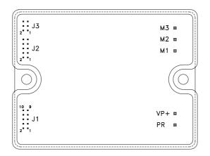
Figure 3-3: Raven Connector Locations
